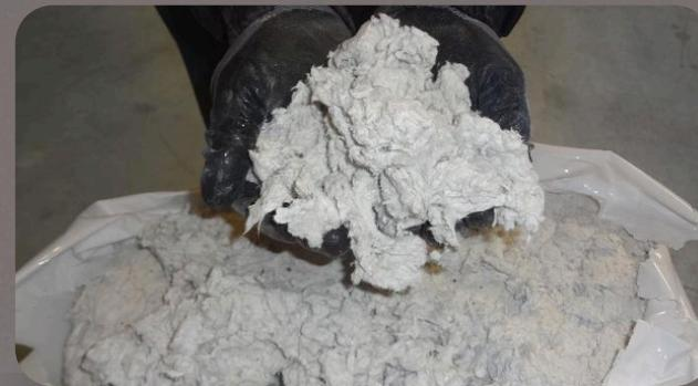
If thermal protection of hot surfaces of steel structures is required, SLMW, a cementitious compound based on sprayed mineral wool, is specially designed to provide thermal protection inside buildings. It is available in HT-GRADE (high temperature) quality.
